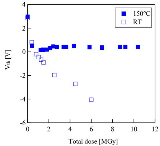
Fig. 2 Total dose dependence of the  $V_{th}$  for SiC MOSFET irradiated at 150°C (filled) and RT (unfilled).
