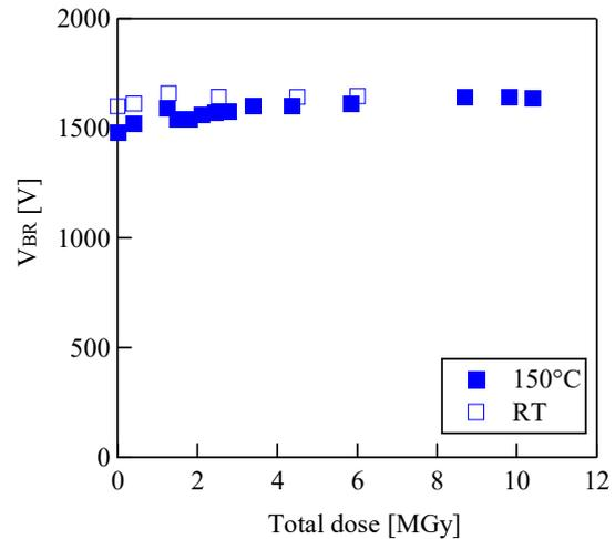
Fig. 5 Total dose dependence of the  $V_{BR}$  for SiC MOSFET irradiated at 150°C and RT.
