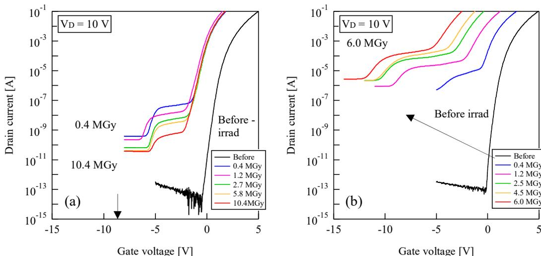
Fig. 1  $I_D$  vs  $V_G$  curves in the subthreshold region for SiC MOSFET before and after irradiation at (a) 150°C and (b) RT.
