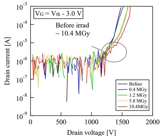
Fig. 4 Blocking characteristics of SiC MOSFET before and after irradiation at 150°C.
