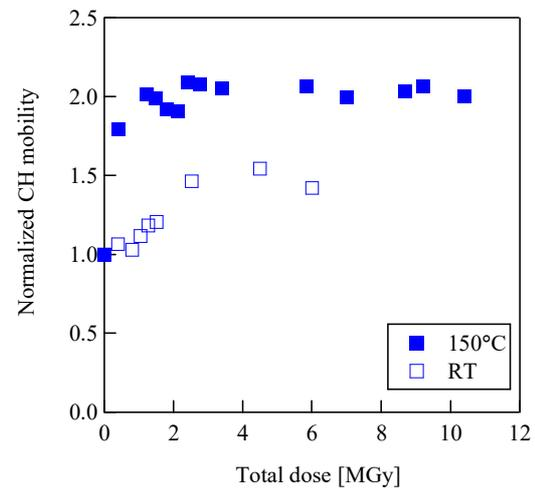
Fig. 3 Total dose dependence of the  $\mu_n/\mu_{n0}$  for SiC MOSFET irradiated at 150°C (filled) and RT (unfilled).
