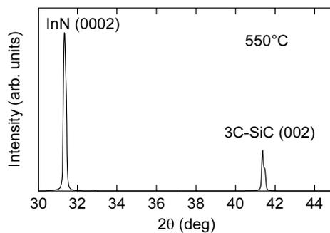
**Fig. 2** Typical  $\theta$ - $2\theta$  XRD profiles of hexagonal InN grown on a 3C-SiC (001) substrate.
