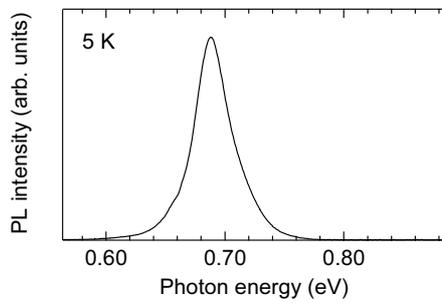
**Fig. 5** Photoluminescence spectrum of hexagonal InN grown at 550 °C.
