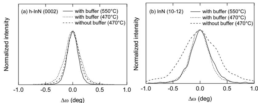
**Fig. 4** XRD rocking curves for (a) hexagonal InN (0002) and (b) hexagonal InN (10-12).
