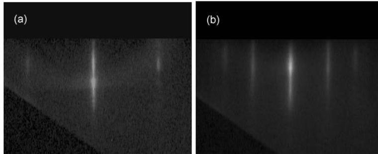
**Fig. 1** RHEED patterns of h-InN grown on 3C-SiC (001) (a) with and (b) without a buffer layer observed at the 3C-SiC  $\langle 110 \rangle$  azimuth.
