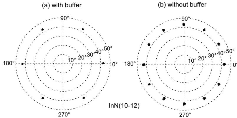
**Fig. 3** XRD pole-figures of (10-12) h-InN grown (a) with a buffer layer and (b) without a buffer layer.
